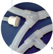
Manifolds are manufactured by molding straight sections of tubing or hose with connectors such as T's and Y's. Molded connectors provide a seamless transition for a continuous, unrestricted flow.
